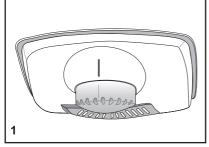
Operating temperatures are controlled by the thermostat (see diagram) located on the ceiling of fridge compartment. Settings may be made from min to max, max being the coldest position.
